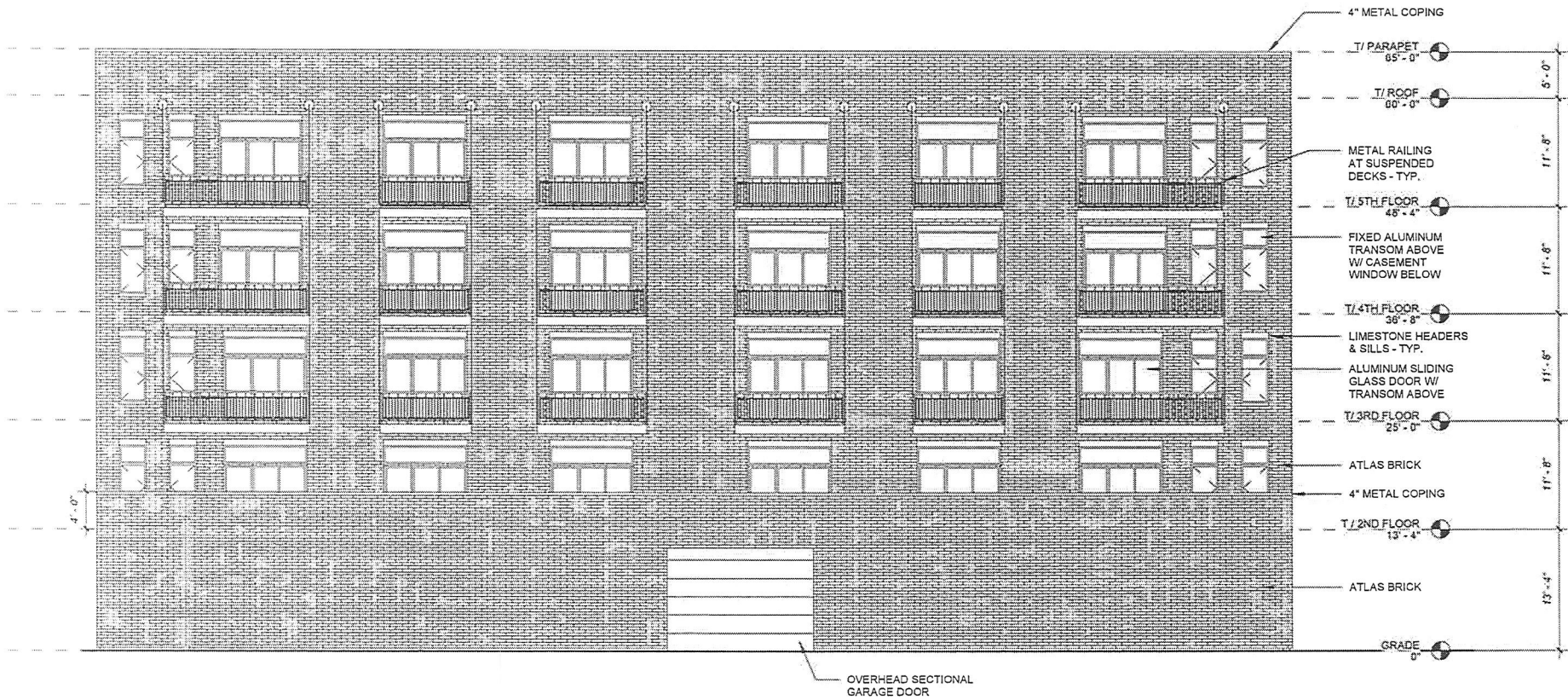
1 SOUTH ELEVATION SCALE: 3/32" = 1'-0"
