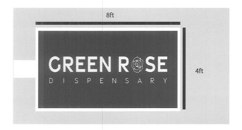
12" Wide Extruded Aluminum — Sign Frame with 2" Wide Perimeter Face Retainers
